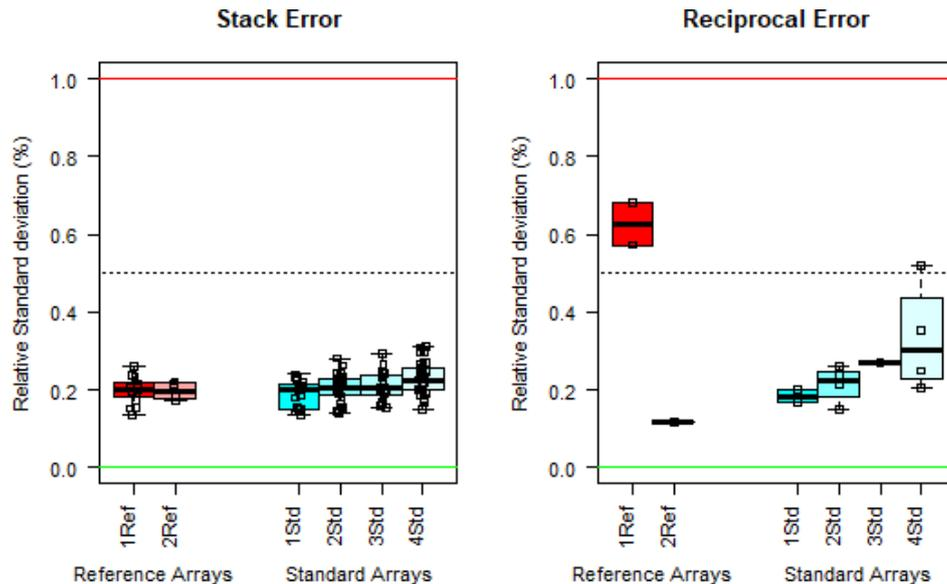
**Figure 4** Result of test measurements with sample container filled with tap water. Abbreviations on the x-axis refers to labels in Figure 3
